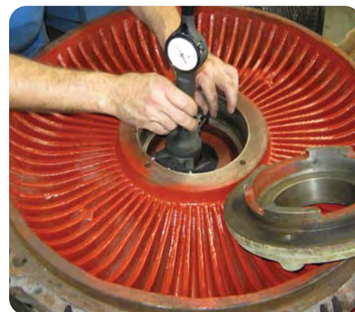
Precision, multi-point fits are taken with bore gauges
